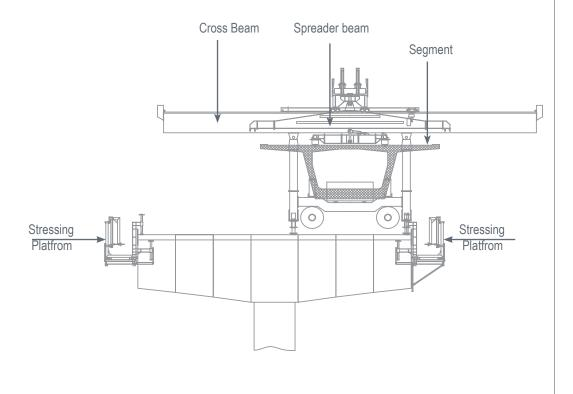
High erection rate up to 2 pairs of segments per shift
